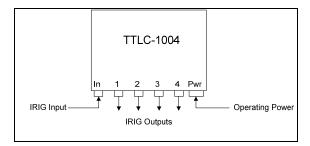
Note that in the above diagram all IRIG outputs are isolated from ground and are "floating". The IRIG input is not isolated from ground.
