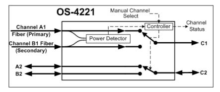
The OS-4221 switch will go in a bypass state under any of the following conditions:
