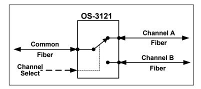
The OS-3121 switch will go into the B=C state under any of the following conditions:
