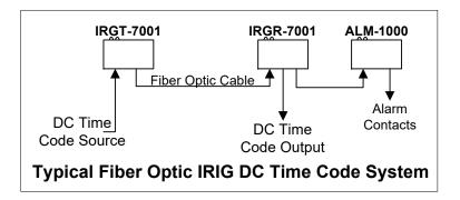
Both should be connected as shown and a DC time code signal applied to the transmitter. The receiver will reproduce this signal with no adjustments.
