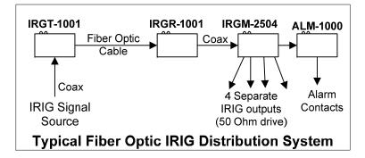
The IRGM-2504 provides four electrical outputs. Multiple IRGM-2504 units may be "daisy-chained" when more than 4 output channels are required.
