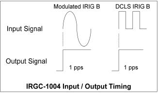
Note that the 1 pps pulse is synchronized with the leading edge of every data and position bit, not necessarily with the reference bit.
