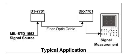
The DT/DR-7701 is an analog transmission system. All signals on the bus that are less than 5 volts pp will be transmitted linearly. Any signal from5 volts to 20 volts pp will be compressed but transmitted for monitoring purposes clamped to 5 volts.
