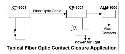
Note that when TTL inputs are used, a logic 1 signal signifies a contact closure and a logic 0 signal signifies an open contact. Also note that the CR-8001 receiver output contacts are fully isolated from each other and any other terminal.
