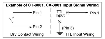
\*Note that the output contacts are only capable of switching a maximum of 0.5 Amperes resistive at 125VAC or 1.0 ampere resistive at 24 VDC and are isolated from the housing and all other pins.
