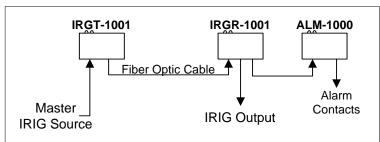
Typical Fiber Optic IRIG Sine Wave System
